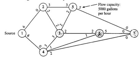
Due to the varying pipe sizes, the flow capacities also vary. By selectively opening and closing sections of the pipeline network, the firm can supply any of the storage locations.
